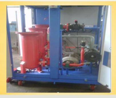
The Particle removal System (NAS Oil filtration System) removes the solid Particles present in Oil. It is combination of very Fine filtration with high flow depend on drain valve size to remove solid particulate contamination. Plant is designed for removing the fine solid contamination and to polish the oil to achieve Oil Cleanliness level: ISO 4406 and NAS 1638. Number of pass depend on inlet cleanliness level of oil.
